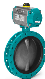
Desponia® - U-section Centric butterfly valve with loose NH liner or FPM VD liner U-section Ductile iron DN150-1600 With any type of actuation
