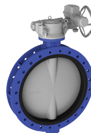
Series 820/20 Centric butterfly valve with loose NBR liner U-section Ductile iron DN150-1600 With any type of actuation
