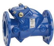
Series 41/60 Swing check valve with free shaft end Resilient seated Ductile iron DN50-300
