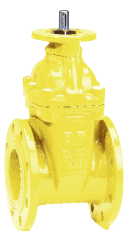
Series 15/78 Flanged gate valve with ISO top flange Short face to face DIN F4 NBR wedge Ductile iron DN50-400
