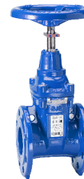
Series 06/35 Flanged gate valve with position indicator and handwheel Short face to face DIN F4 NBR wedge Ductile iron DN50-400
