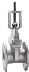
Series 06/46 Flanged gate valve with rising stem (OS&Y) Short face to face DIN F4 NBR wedge Duplex stainless steel DN40-200
